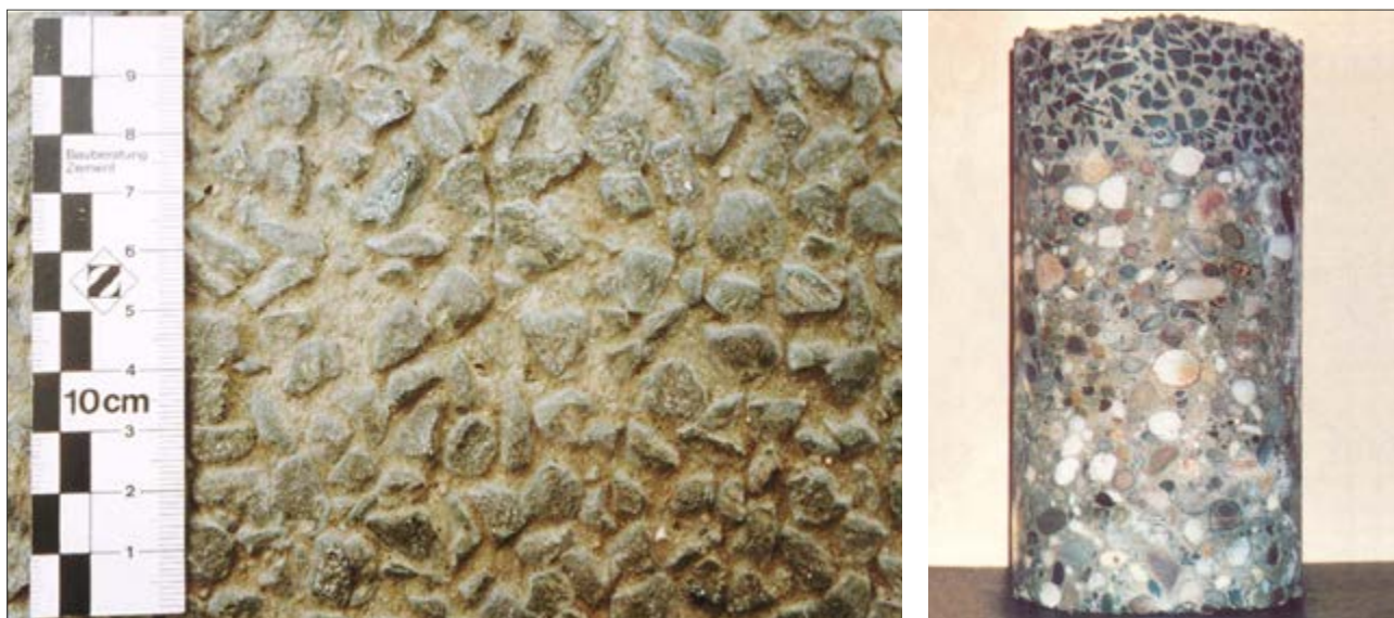
Figure 4.28 Exposed Aggregate Surface and Core Showing Two Layer Construction
